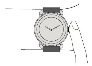
Power On/Off: Press and hold the crown for 3 seconds.
