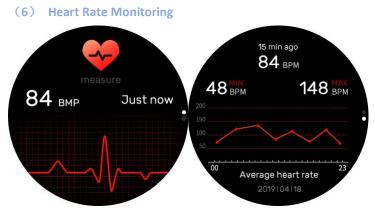
A. Watch: Go to heart rate monitoring interface, automatically start real-time measurement, measurement results will be displayed in 20 seconds. Scroll up to see heart rate details.
